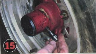
Rotate the wheel/hub until the hole is at 4:00 designation. This will allow the excess fluid to drain off, leaving you with the proper fluid amount. Once it stops draining, reinstall the drain/fill plug
