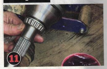
Designate the proper wheel bearings against the hub bearings. The hub bearings are slightly smaller and won't slide all the way on the axle like our wheel bearing. These two larger ID bearings will get packed with wheel bearing grease, and they can be installed onto the axle, or set into the race in the strut.
