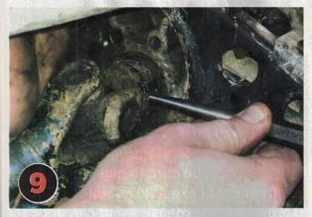
Use a hammer and punch to drive out the drift pin that secures the axle knuckle onto the splined output shaft. It will be difficult as there is not much space, rotate the axle until it is designated to where you have room for the hammer.
