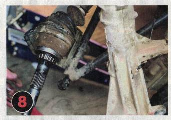
With the strut separated from the a-arm, pull the cv axle out of the strut. That bearing is the inner cv/strut wheel bearing. It will get greased and reused, or you can replace them with new from East Lake Axle. Ours did not show any wear, but if you opt to replace it, you will need to remove and replace the bearing races from the strut as well.
