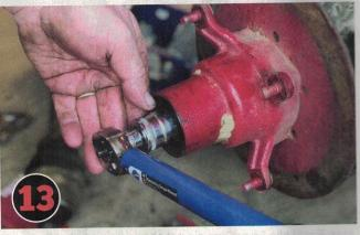
Carefully slide the hub/clutch bearing assembly from step 5 onto the new axle. Then install the hub onto the shaft and install the outer hub bearing. These do not get greased. The new axle comes with a different style nut and a cotter key instead of the circlip retainer. The torque spec is very low at 165 IN lbs., or just under 14 ft. lbs. Do not over-tighten or you will ruin your bearings.
