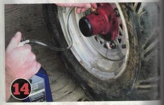
Push the hub oil cap into place, Re-assemble the entire suspension system in the reverse of taking it apart. You are ready to refill the hub with oil. Polaris recommends only using their Demand Drive Plus Fluid, but we've heard that Type F transmission fluid will work as well. The fill plug is removed a 3/16 Allen, and then fill the hub with the oil hole at 12:00.
