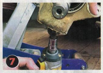
Remove the lower strut nut that attaches it to the a-arm. We used an impact, because it can spin, but it can be done without. Once removed, you will want to use a pry bar to apply downward pressure on the arm. You can smack it with a hammer if it won't separate.
