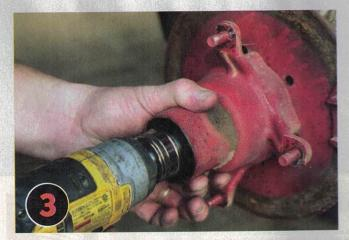
Remove the large castle nut from the end of the axle. We used an impact gun, but if you don't have one, you can hold the inner axle from spinning with pliers or vise grips.
