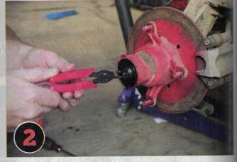
With the hub oil drained into a pan or towel, remove the snap ring from the end of the axle with a pair of snap ring pliers. You will also need to remove the two brake caliper bolts, and hang the caliper out of the way.
