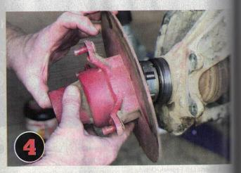
Remove the hub assembly, being careful to keep the outer bearings in the hub. You can take them out for inspection, cleaning etc., but you will want to pay special attention to the order.
