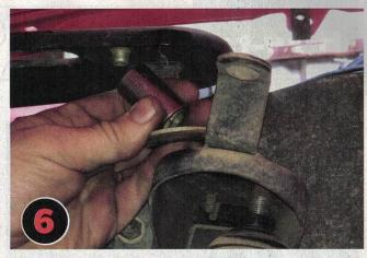
Remove the top nut from where the strut attaches to the frame. Pay attention to the washer placement. You could probably do this project without removing this nut, but it gives you extra room to move everything around.
