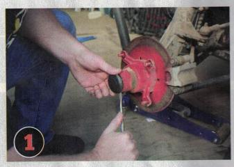
Pressure wash any mud from the front hub/a-arm area, secure the machine on a jack or a stand, and remove the front wheel. You can use a flat blade screwdriver to remove the hub oil cap. It will have sealing O-rings, and oil should drain when you pop it out.
