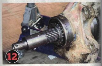
With the new cv installed through the strut and inner bearing, yo will then grease and install the outer strut/wheel bearing. These get packed with grease, but the slightly smaller hub bearings are lubricated by the hub oil.
